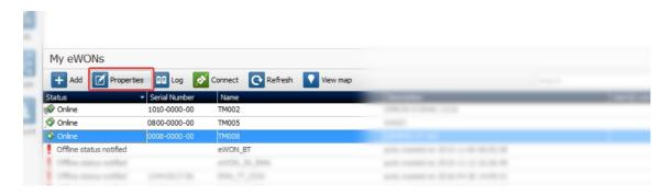
Once in the Properties of the targeted eWON, configure the LAN Devices & Firewall.
