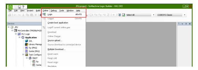
A new interface show up, displaying the possible connection. The PLC discovery is already in action.
