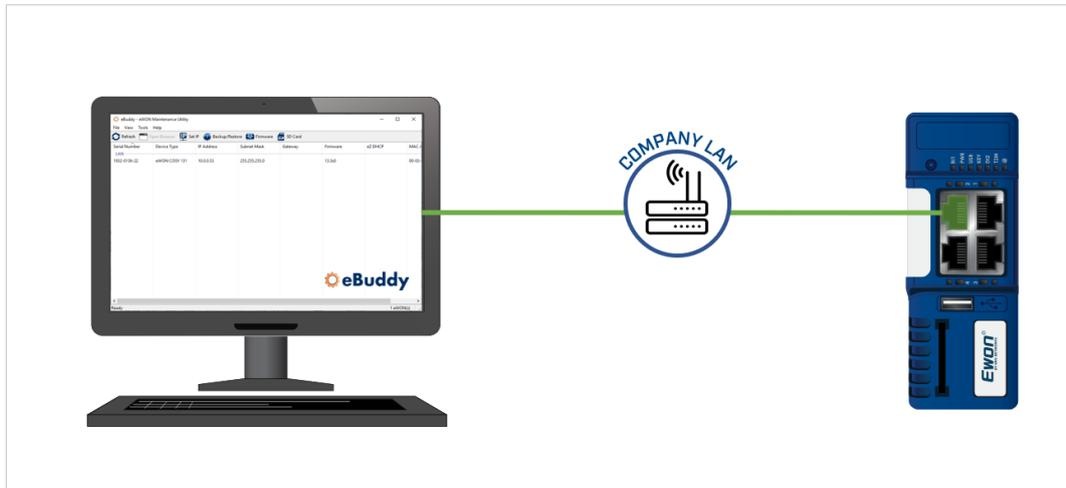
Fig. 26 Connect the computer indirectly to the Ewon though Company LAN
