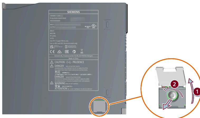
Figure 4-1 Removing the screw for functional grounding
