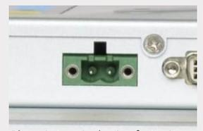
Phoenix terminal using fastening type power connector
