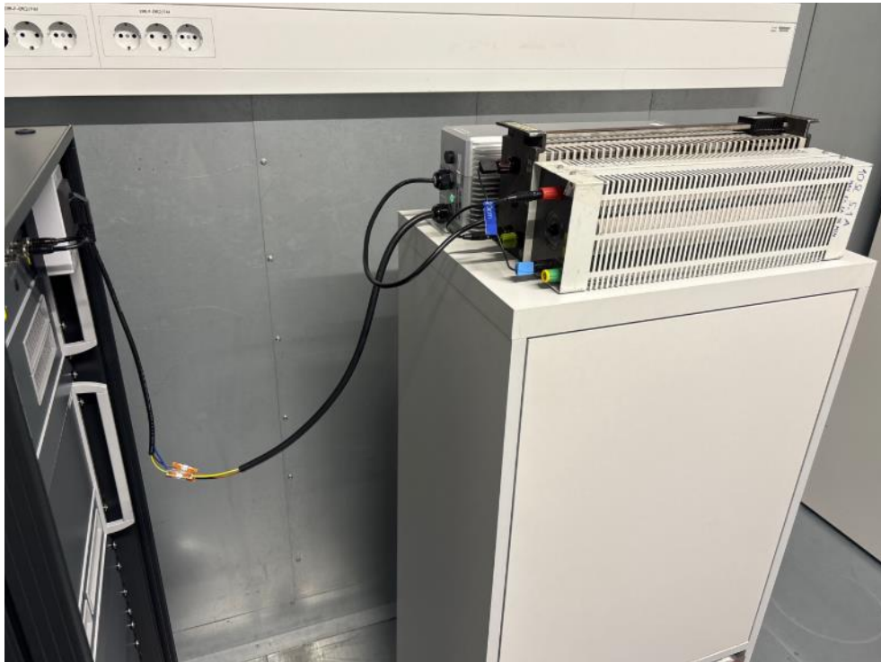
Figure 8: Harmonic current emissions measurement
