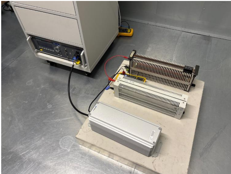
Figure 24: Electrical fast transient/burst immunity test
