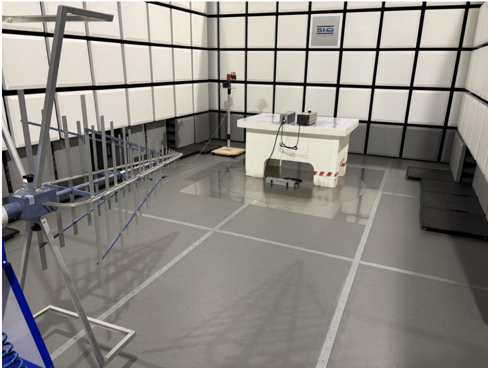
Figure 3: Radiated emission measurement
