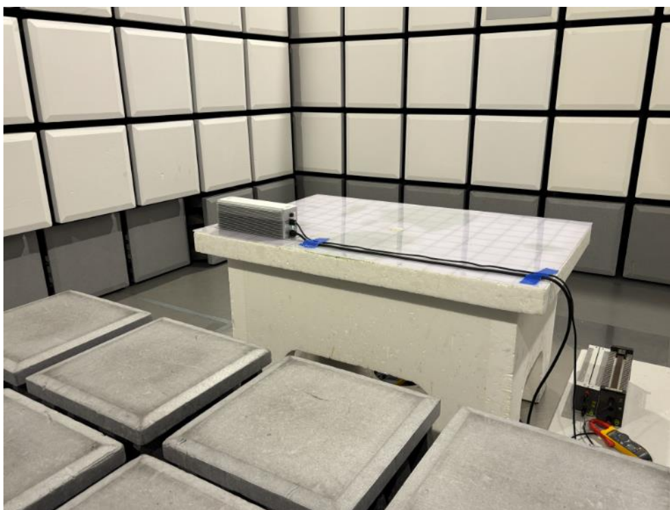
Figure 22: Radiated, RF electromagnetic field immunity measurement
