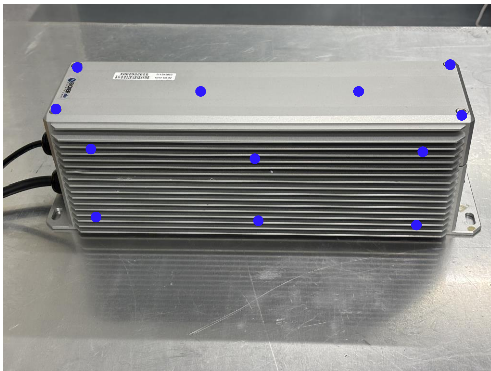
Figure 13: Electrostatic discharge immunity test
