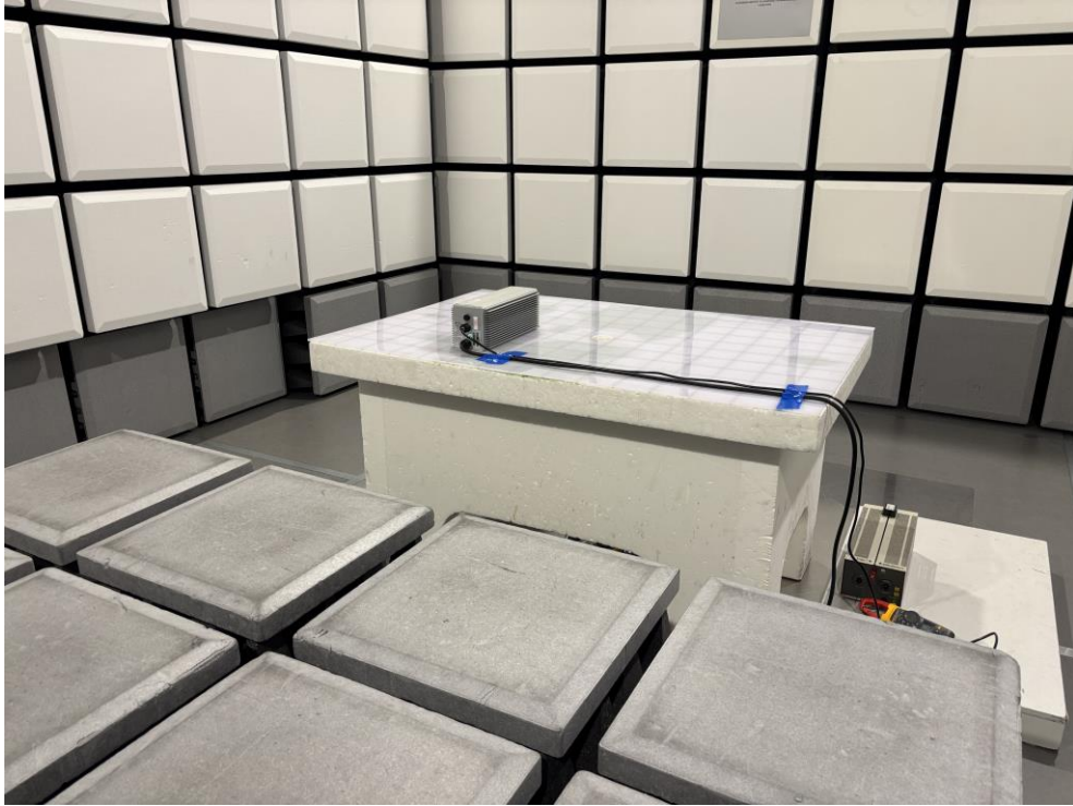
Figure 21: Radiated, RF electromagnetic field immunity measurement
