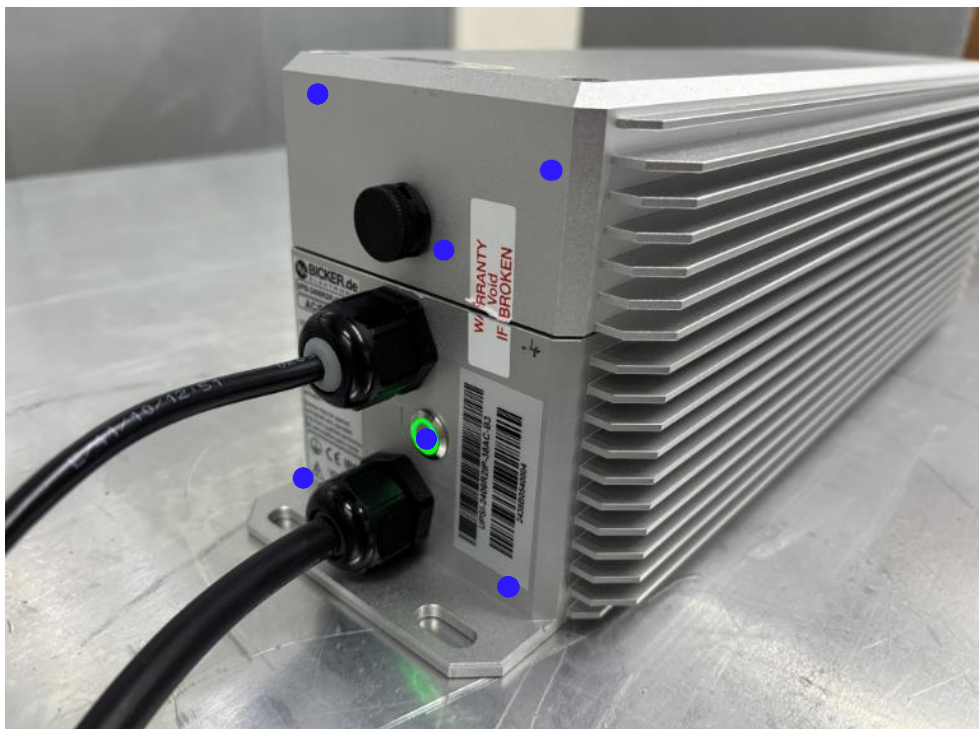
Figure 18: Electrostatic discharge immunity test
