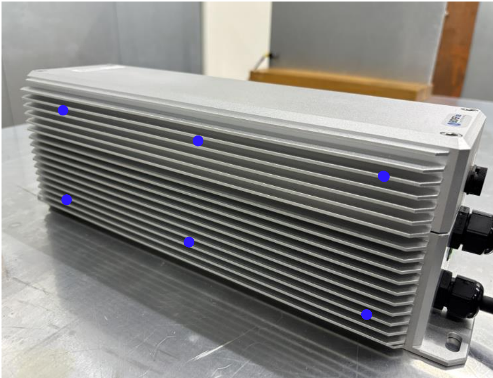
Figure 19: Electrostatic discharge immunity test
