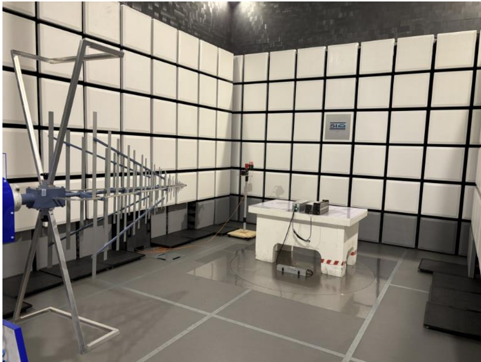
Figure 5: Radiated emission measurement
